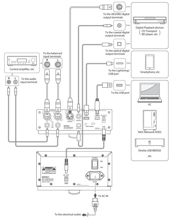
\* Depending on the control amplifier used, there may be a caution regarding simultaneously connecting RCA and XLR, so refer to the operation manual of the respective control amplifier.
